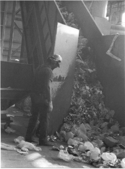
At Rumpke's Material Recovery Facility in Dayton, commingled recyclables from Darke County go up the conveyor belt to be sorted
